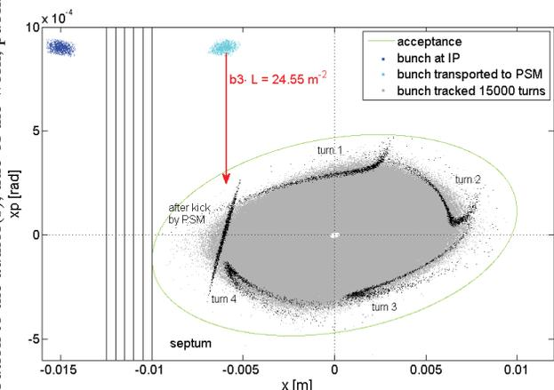
Figure 2: Multipole kicker injection of a bunch from the booster on SLS 2.0.
