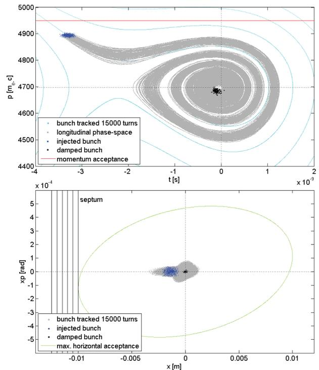
Figure 1: Longitudinal injection of a bunch from the booster on SLS 2.0 assuming an RF frequency of 100 MHz. Up: longitudinal phase space. Down: transverse horizontal phase space.
