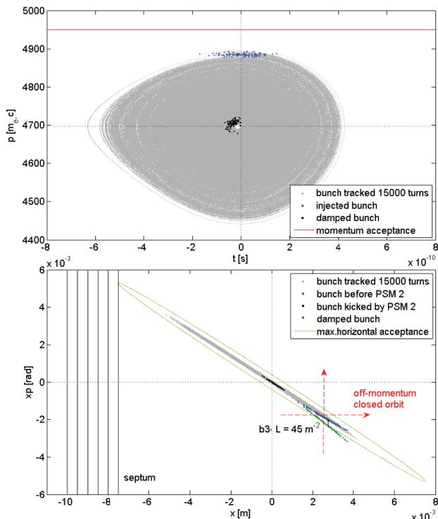
Figure 3: Off-momentum multipole kicker injection of a bunch from the booster on SLS 2.0. Up: longitudinal phase space. Down: transverse horizontal phase space.
