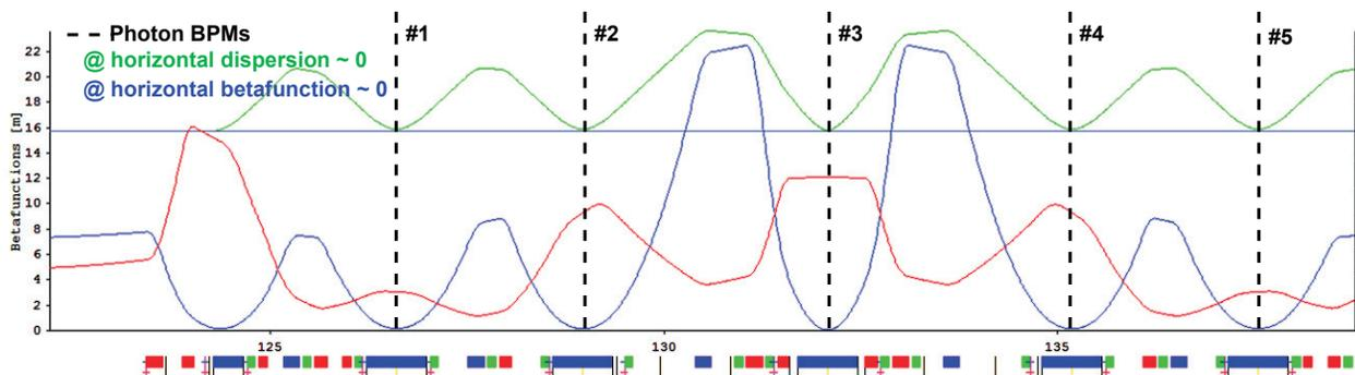
Figure 1: One arc section of the SLS-2 lattice (Version AD05F) with a schematic view of the magnets at the bottom (dipole magnets in blue) and the optical functions. The horizontal beta function (blue) and the horizontal dispersion (green) vanishes in the center of the bending magnets in order to provide small horizontal emittance. Five additional photon BPMs (#1-#5) have been added in the center of the main bends for improved orbit sampling.
