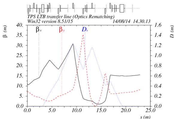
Figure 6: The beam optics of LTB with the launching conditions at the linac exit calculated by fitting the measured beam sizes.
