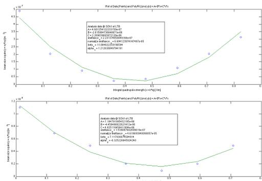
Figure 5: Beam size variation with quadrupole scan and data fitting.
