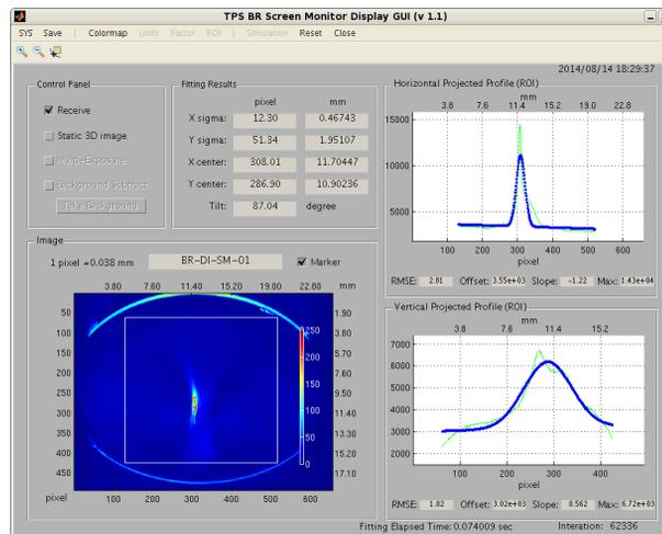
Figure 7: Electron beam appears at the first screen monitor of booster located at the exit of injection kicker.
