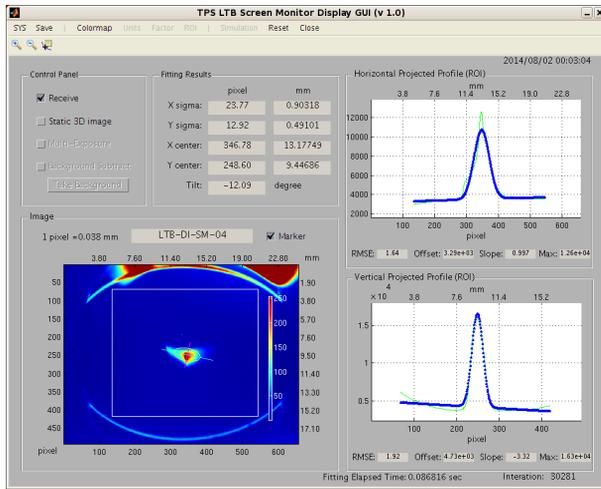
Figure 4: Beam profile at the end of LTB.
