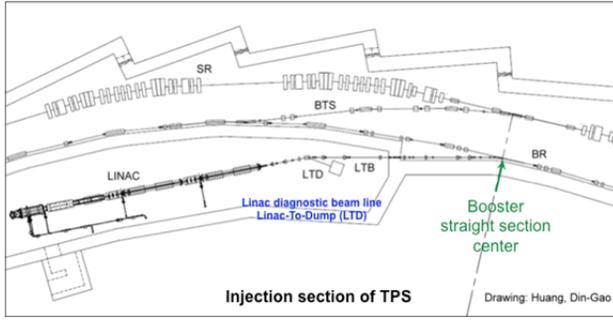
Figure 3: Layout of TPS injection sections of booster and storage ring including linac, LTD, LTB, and BTS.
