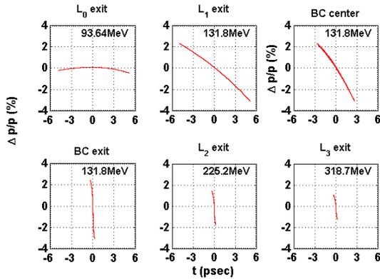
Figure 3: Evolution of longitudinal phase space through the beamline.
