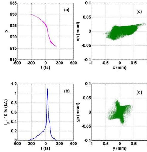
Figure 4: The (a) longitudinal phase space (b) current profile (c), (d) transverse (x and y-plane) phase space of electron distribution at the  $L_3$  exit.
