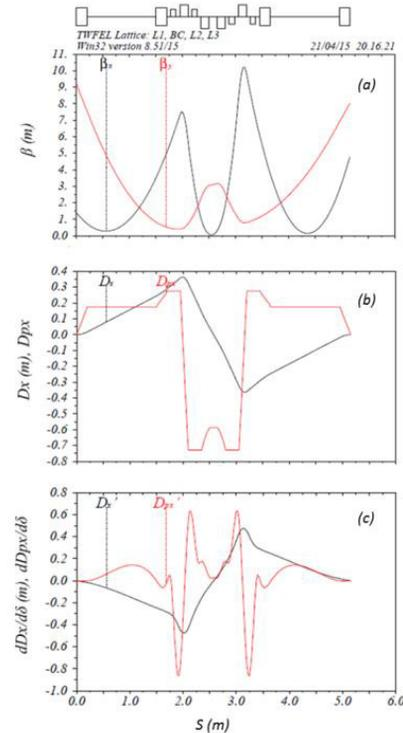
Figure 2: Optics of the bunch compressor: the evolution of the (a) betatron function (b) first order dispersion ( $R_{16}$  and  $R_{26}$ ) (c) second order dispersion ( $T_{166}$  and  $T_{266}$ ) in the compressor.
