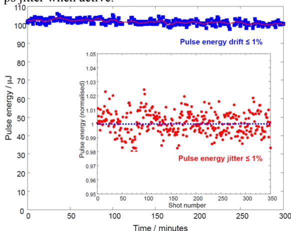
Figure 5: Laser pulse energy variation delivered by the VELA photoinjector laser and transport system to the photocathode, measured over a typical operating period of six hours (main figure, blue; 10 minute average, red) and over 350 shots (at 10 Hz). Both the long and short variation is within 1 % of the pulse energy.
