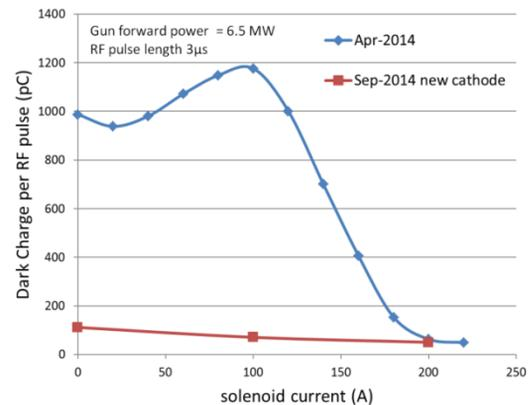
Figure 3: DC measured on WCM-01 with the original (April 2014) and new (Sep 2014) photocathode.
