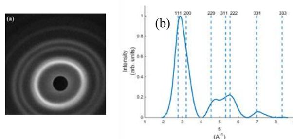
Figure 6: (a) 1000 shot accumulated diffraction pattern of polycrystalline platinum, and (b) Azimuthal integration of polycrystalline platinum diffraction with expected diffraction peaks overlaid as dashed lines.
