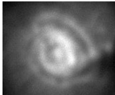
Figure 1: Beam image with rings attributed to machining marks on cathode.
