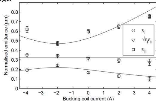
Figure 2: Measured (points) Eigenmode emittance with bucking coil current and theory (lines)
