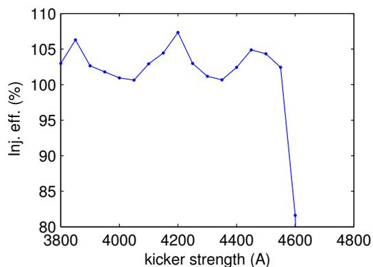
Figure 4: Injection efficiency vs. kicker amplitude.
