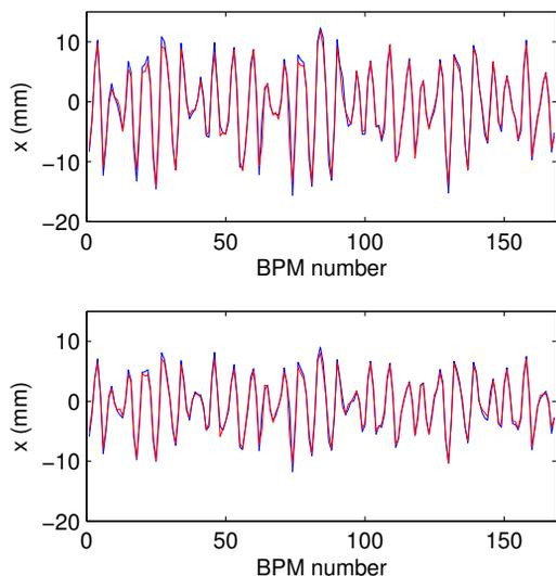
Figure 5: Measured trajectory of the injected beam during the first turn of the storage ring (blue) compared to the reconstructed model trajectory (red). Top: Kickers at 3800 A. Bottom: Kickers at 4550 A.
