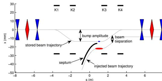
Figure 1: Injection schematic for the Diamond storage ring.
