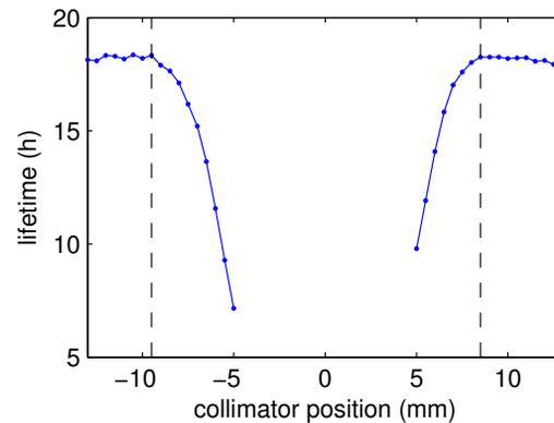
Figure 3: Lifetime vs. horizontal collimator aperture. The dashed vertical lines indicate the point at which the collimators begin to affect the lifetime.
