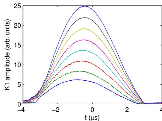
Figure 6: Kicker 1 pulses measured between 1000 A and 5000 A.
