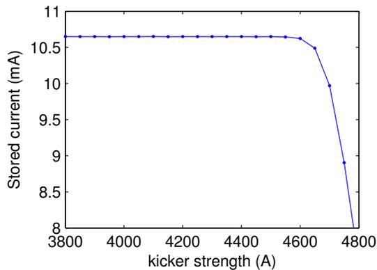
Figure 2: Stored current vs. injection kicker amplitude.
