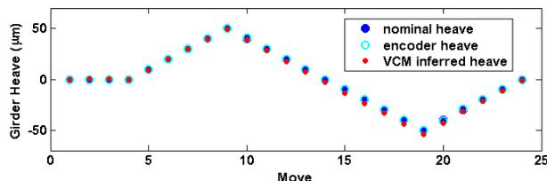
Figure 5: C6G2 heave scan: (blue dots) nominal imparted heave, (cyan circles) heave from remote control encoder readings, (red dots) girder heave inferred from the variation of the vertical steerers.
