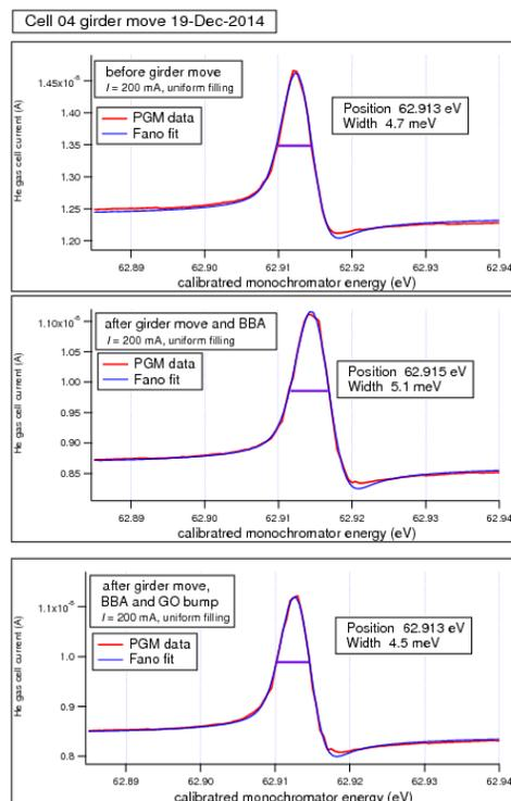
Figure 3: Energy calibration of the PGM beamline system. (Top) initial setting, showing a Helium photo-ionization peak at 62.913 eV and a full width of 4.7 meV. (Middle) after cell-4 is realigned the peak is shifted to 62.915 eV with a width of 5.1 meV. (Bottom) the configuration is perfectly restored when GO=239  $\mu\text{m}$  is implemented at BPM(4,7).
