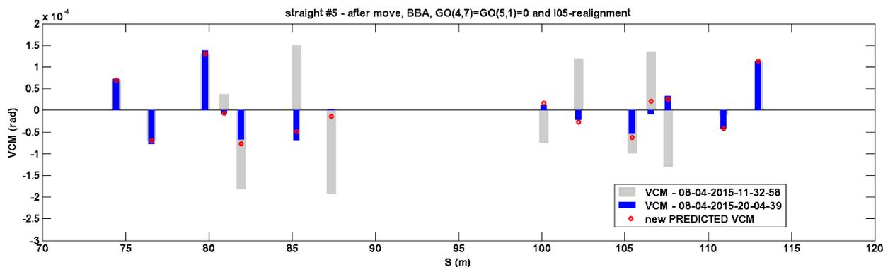
Figure 4: VCM strength reduction after C5G1G2 realignment and the removal of GO(4,7) following the full realignment of I05 beamline. The new VCM pattern in the machine (blue bars) agrees well with model predictions (red dots).
