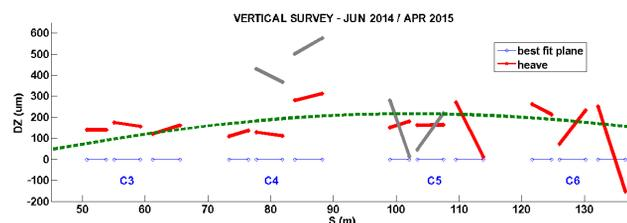
Figure 1: Vertical survey of the Diamond Storage Ring. The red segments join the monuments at girder edges, showing the present situation after the realignment of straight-05, while the gray ones show the state of the machine before it. The dashed green line is a fit to the 148 monument levels, which is used as realignment baseline (see text).
