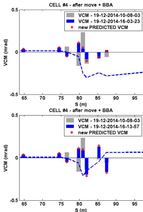
Figure 2: Vertical corrector changes after realignment of cell 4 and four BBA cycles (top) and with the introduction of a GO(4,7)=239  $\mu\text{m}$  to make the move transparent (bottom). (Gray) initial set of correctors, (blue) new corrector pattern, (red dots) predicted VCM strengths. The change in total corrector strength (dashed blue line) becomes positive after the introduction of a GO.
