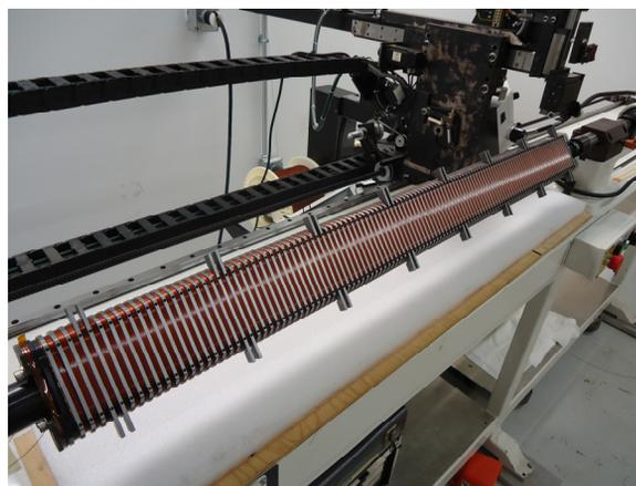
Figure 1: SCU1 magnet core on winding machine.
