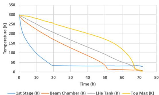
Figure 2: The SCU1 temperatures during cool down.
