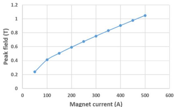
Figure 4: SCU1 magnet excitation curve.
