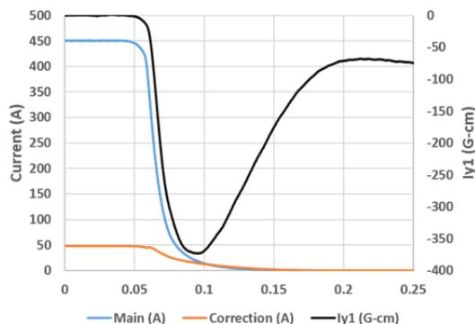
Figure 7: Change of the SCU1 magnet currents and the first vertical field integral during magnet quench.
