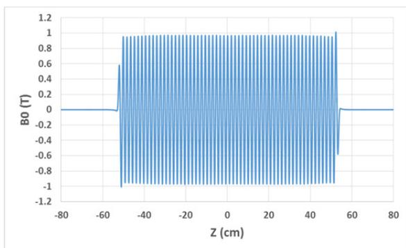
Figure 5: Measured field profile at design current of 450A.
