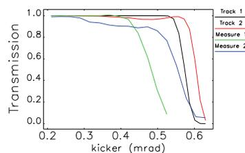
Figure 5: Comparison of kick aperture. Black: simulation of operation lattice; Red: simulation of tweaked lattice; Green: measurement of operation lattice; Blue: measurement of tweaked lattice.
