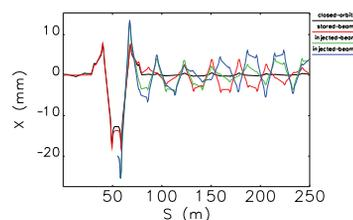
Figure 2: Beam trajectories for injection. Black: stored beam, closed bump. Blue: injected beam, closed bump. Red: stored beam, non-closed bump. Green: injected beam, non-closed bump. The septum magnet is at 56 m.
