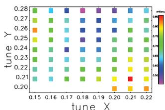
Figure 6: Injection efficiency color map (range from 50% to 85%) on fractional betatron tunes space.
