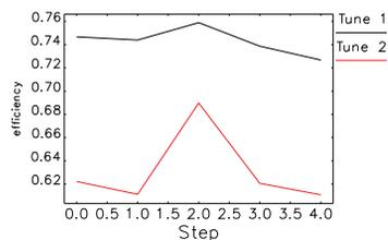
Figure 7: Injection efficiency at tweaked (black) and original tunes (red), repeated for 5 times.
