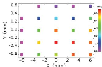
Figure 4: Injection efficiency as a function of stored beam orbit at ID4. Measurements on RHB lattice.
