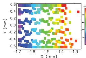
Figure 3: Beam-based measurement of the septum magnet position relative to stored beam. Color map showing the beam lifetime measured in minutes (5 to 500 minutes).
