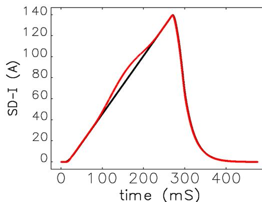
Figure 1: SD magnet new non-linear (Red) and original linear (Black) ramps.
