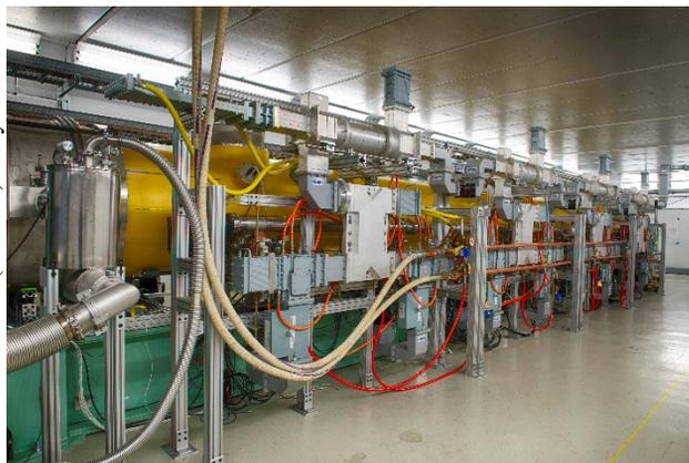
Figure 2: CM2 with waveguide distribution system.
