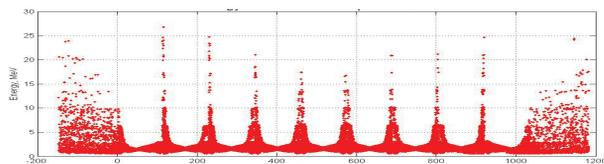
Figure 2: Distribution of energy of particles lost in cavity as function of impact  $z$ -coordinate.
