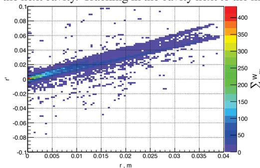
Figure 8: Transverse phase space distribution of DC particles exiting from the 125 GeV quadrupole.
