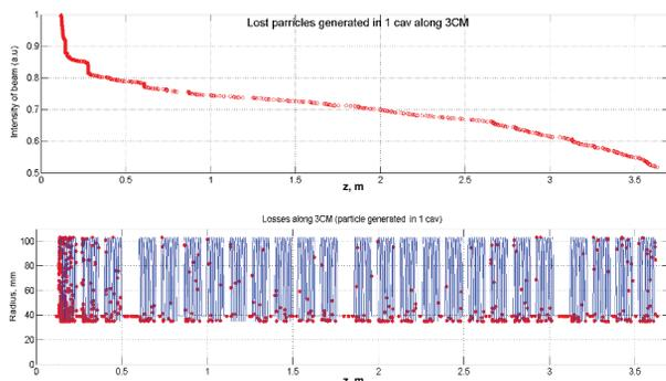
Figure 6: Losses along string of the cavities.
