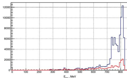
Figure 9: Energy distribution of DC electrons at the exit of 125 GeV quadrupole. In red histogram tracks are weighted with  $W_{FN}$  weights.
