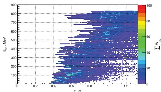
Figure 7: Energy distribution of losses as a function of  $z$ -coordinate of impact in the 125 GeV quadrupole.
