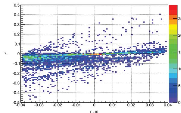
Figure 4: Transverse phase space distribution for electrons leaving emitting cavity. Color scale corresponds to the energy in MeV.
