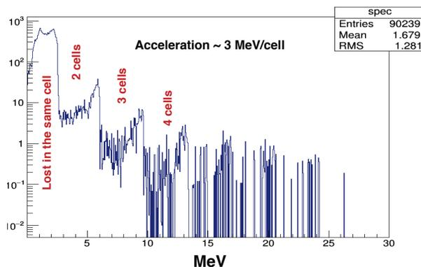
Figure 3: Energy spectrum of particles lost inside cavity.
