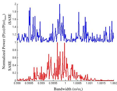
Figure 5: After the initial phase shifters, the radiation spectrum appears to have become a frequency comb, in which certain resonances have been amplified due to a large phase shift early in the FEL process.
