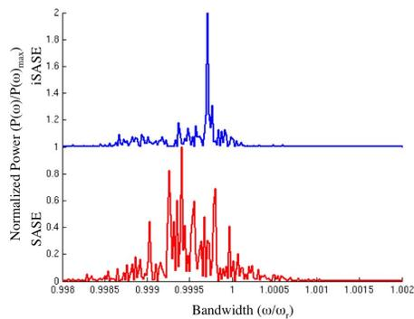
Figure 4: The radiation bandwidth at the end of the FEL process for case B shows a peak near the target radiation frequency in the iSASE spectrum, as compared to the less sharp SASE spectrum. The RMS bandwidth of this solution is about 4.32 times smaller than the SASE bandwidth.
