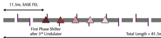
Figure 1: The base-lattice layout for the simulated FEL; the first phase shifter was placed after the third undulator, with focusing and defocusing quadrupoles maintaining the beam optics through the FEL.
