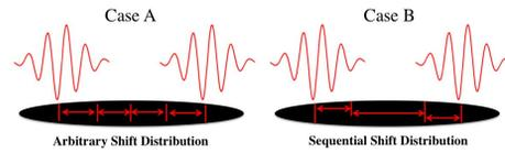
Figure 2: For case A, each phase shifter initially provided the same shift:  $3 l_{\text{slip}}$  for  $l_{\text{slip}} = 290 \lambda_r$ . For case B, the initial phase shifter settings varied in a geometric sequence in which the five shifters provided  $16 l_{\text{slip}}$ ,  $8 l_{\text{slip}}$ ,  $4 l_{\text{slip}}$ ,  $2 l_{\text{slip}}$ , and  $1 l_{\text{slip}}$  shifts respectively.
