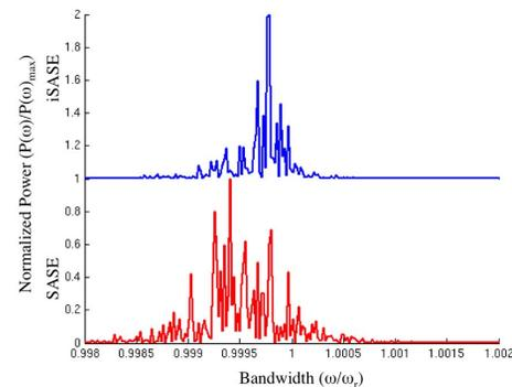
Figure 3: The radiation bandwidth at the end of the FEL process for case A shows a peak near the target radiation frequency in the iSASE spectrum, as compared to the less sharp SASE spectrum. The RMS bandwidth of this solution is about 4.42 times smaller than the SASE bandwidth.
