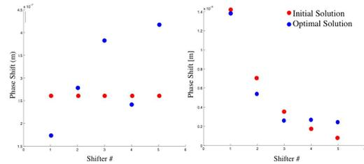
Figure 6: The initial and optimal phase shifter settings for case A (left) and case B (right) show that, in both cases, the total shift provided needed to be increased, and that the order of the provided shifts should not be arbitrary.
