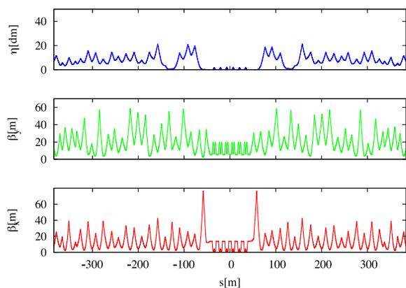
Figure 3: Lattice parameters for the proposed modification. The upgraded sextant is centered at  $s = 0$ .
