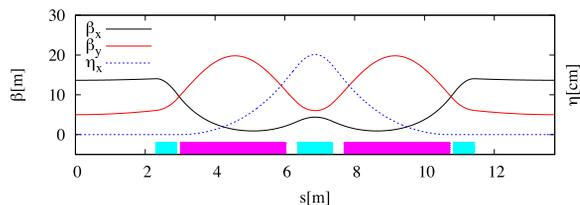
Figure 2: Lattice parameters for one proposed DBA cell. Quadrupoles are shown in cyan, and combined-function dipoles in purple. There are no sextupoles in this sextant of the storage ring.
