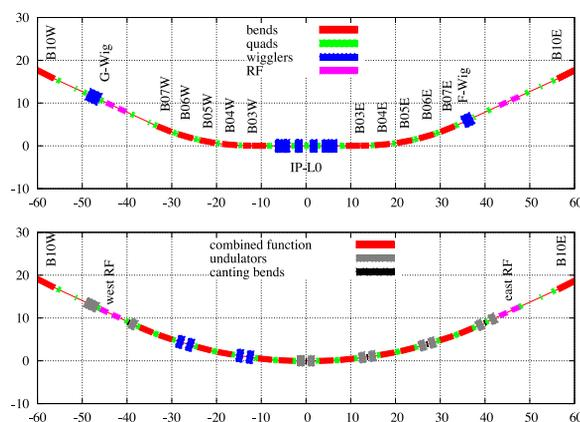
Figure 1: Top: existing user area layout. Bottom: proposed change to user area, removing the CLEO detector straight. All counter-clockwise beam lines will be replaced with clockwise-facing lines, and all beam lines will utilize undulator sources.
