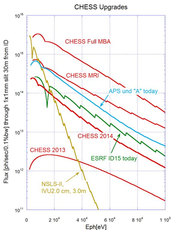
Figure 4: X-ray performance before and after the proposed upgrade. “CHES 2013” refers to the CHES 50-pole wiggler; “CHES 2014” is for the current installation of a 1.5 m CHES Compact Undulator (CCU). “CHES MRI” is this proposal. “CHES Full MBA” is the resulting flux if the remaining 5/6 of the ring (underground, and inaccessible to users) were upgraded to a TME-style arc cell.
