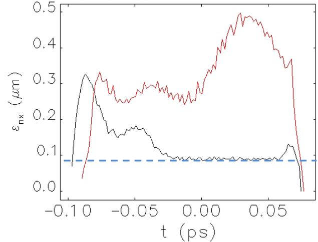
Figure 3: Bend-plane RMS normalized slice emittance for single- (red) and dual-chicane (black) compressors. Incoming beam energy was 250 MeV,  $R_{56} = -0.16m$ . The dashed blue line indicates the pre-compression slice emittance of 0.09  $\mu m$  RMS.
