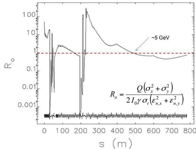
Figure 4: Space-charge impact parameter  $R_o$  vs. distance along the MaRIE linac.  $R_o > 1$  implies space-charge dominated beam transport.
