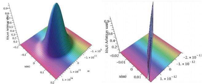
Figure 3 The laser pulse before the Relay optics in  $x-\omega$  (left) and  $x-t$  (right) domains.
