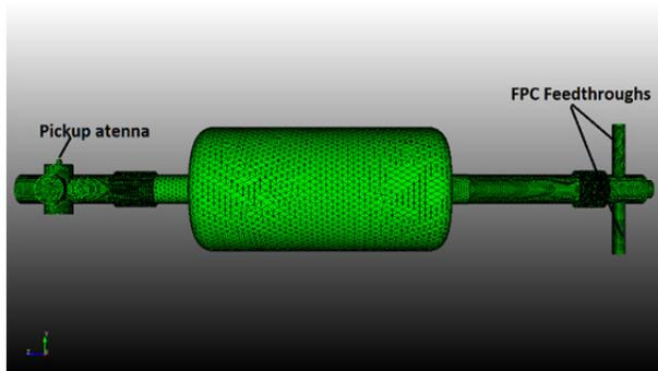
Figure 2: Tetrahedron mesh generated by Cubit with a number of elements equal to 1.5 million.
