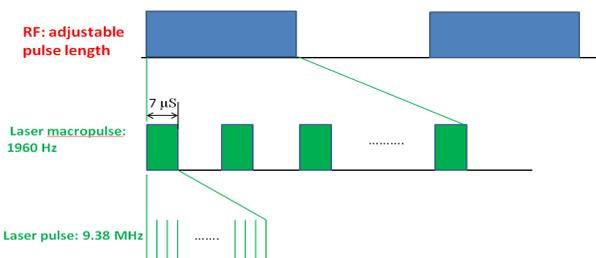
Figure 3: Beam structure of first beam test.
