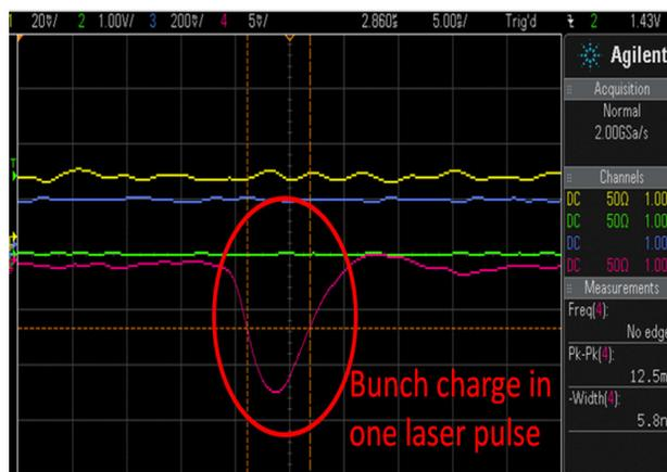
Figure 4: Beam current (top), dark current (middle) and bunch charge (bottom) measured by Faraday Cup.
