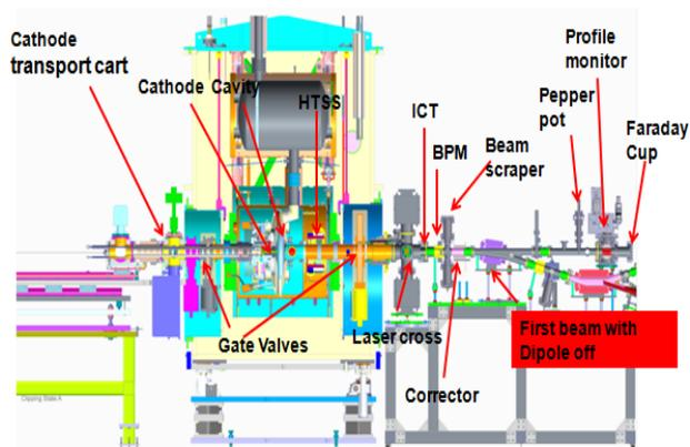
Figure 1: First beam commissioning configuration.
