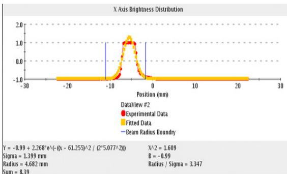
Figure 5: Beam size measured by beam profile monitor.
