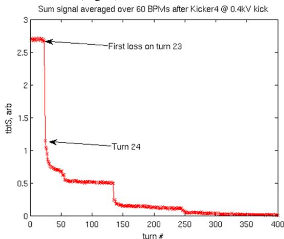
Figure 5: The beam loss as observed from the sum signals of SR BPMs.
