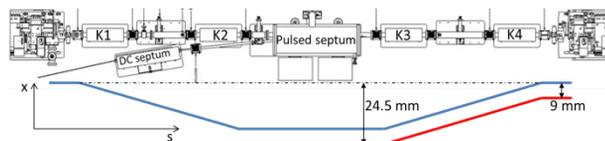
Figure 2: SR injection section and designed injection scheme (red colour represents injected beam, blue colour represents stored beam).
