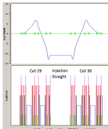
Figure 3: Horizontal DC bump in injection straight section.
