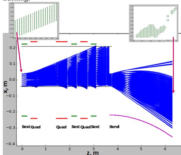
Figure 4: CPS horizontal tracking through the beginning of the long straight and first dipole. Green, red and magenta lines show respective yokes of quads, sextupoles and the dipole. Most beam losses happen in the drifts on the vacuum chamber (grey lines) or photon apertures. The two upper plots show beam trajectories phase spaces at the beginning and at the end of the beamline. For illustration purposes the tracking was performed with only 200 trajectories.
