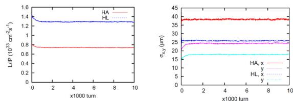
Figure 7: Evolution of luminosity (left) and transverse beam size (right) for two layouts of LHeC, HA and HL.
