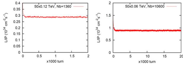
Figure 1: Evolution of luminosity. Left and right plots depict the simulated luminosity for collisions with 120 GeV and 60 GeV  $e^-$ , respectively.
