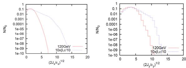
Figure 5: Particle distribution in transverse space for 120 GeV electron beam energy.
