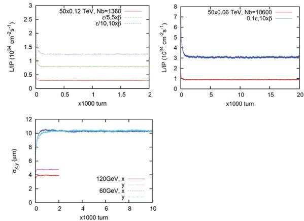
Figure 4: Evolution of luminosity and transverse beam size for ten times higher beta along with  $10\times$  smaller  $\epsilon$ .
