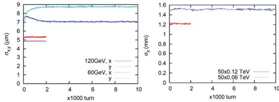
Figure 2: Simulated beam size evolution. The transverse sizes and the bunch length are plotted in the left and right pictures, respectively.
