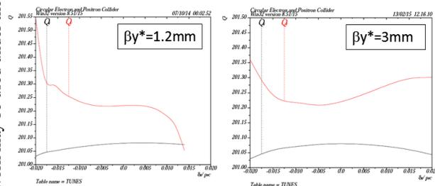
Figure 3: Tune vs. energy deviation.
