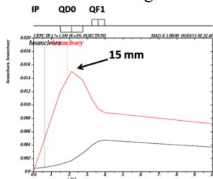
Figure 6: Beam-stay-clear region at the final doublet.
