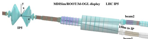
Figure 1: Display of the LHC IP5 geometry. Transverse  $(x,y)$  dimensions were increased by a factor of 100.
