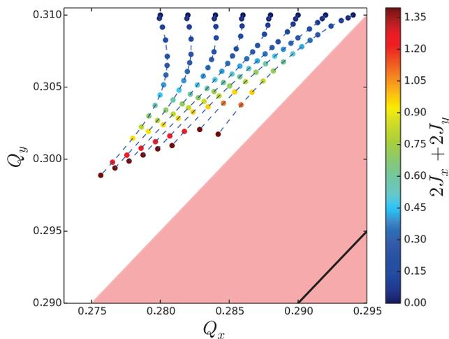
Figure 3: Simulated kicks for different tunes and amplitudes. The vertical kicks ranged from 0.5 mm to 4.5 mm while the horizontal were kept at 0.5 mm. The light red area indicates the linear  $|C^-|$  stopband which was kept at 0.015. The octupoles were kept at nominal powering.
