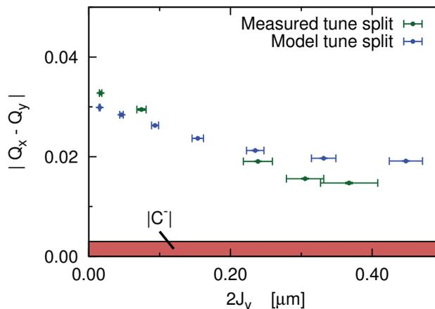
Figure 1: The tune split as a function of the action from the measured data as well as from the simulation based on the nonlinear model of the LHC. The linear  $|C^-|$  was measured during the study and is indicated by the red area.
