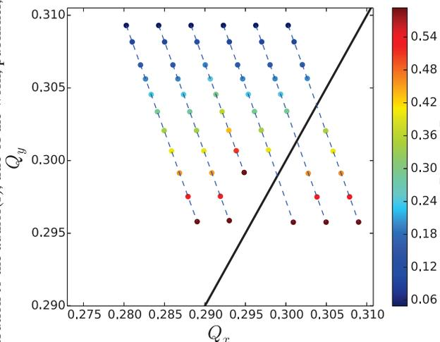
Figure 2: Simulated kicks for different tunes and amplitudes of the vertical kicks. The black diagonal line indicates the resonance  $Q_x = Q_y$ .
