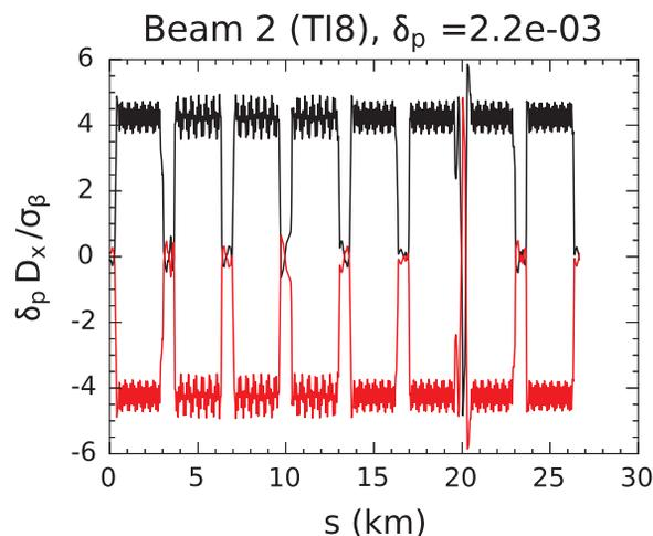
Figure 2: Worst-case off-momentum trajectory in the LHC for beam 2 with a momentum cut of  $\Delta p/p = \pm 0.22\%$  in TI 8.
