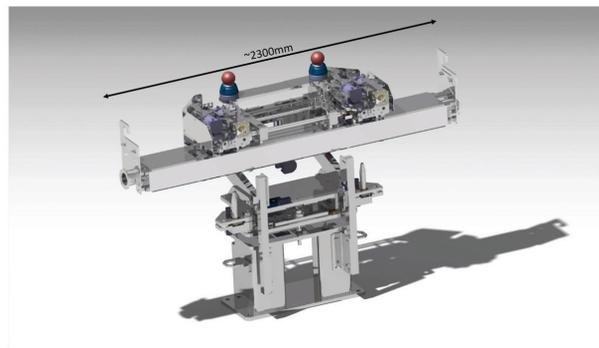
Figure 1: First version of 3D design of LIU transfer line collimator.
