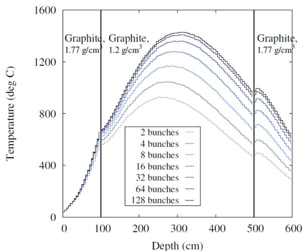
Figure 2: Longitudinal peak temperature profile induced by 50 TeV proton bunches ( $1 \times 10^{11}$ ) in a LHC-like dump core. Bunches are assumed to have a size of  $400 \mu\text{m}$  ( $=1\sigma$ ) and a transverse separation of 1.6 mm.
