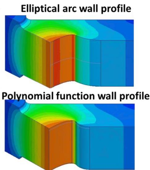
Figure 2: Comparison between elliptical and polynomial wall shape (figures were from HFSS simulations on 1/8 of the middle cell).
