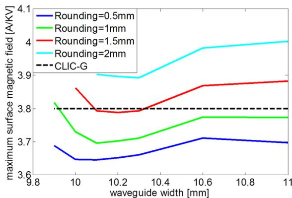
Figure 3: maximum magnetic field versus different roundings and waveguide widths (waveguide opening width in each case fits the requirement of wakefield suppression).
