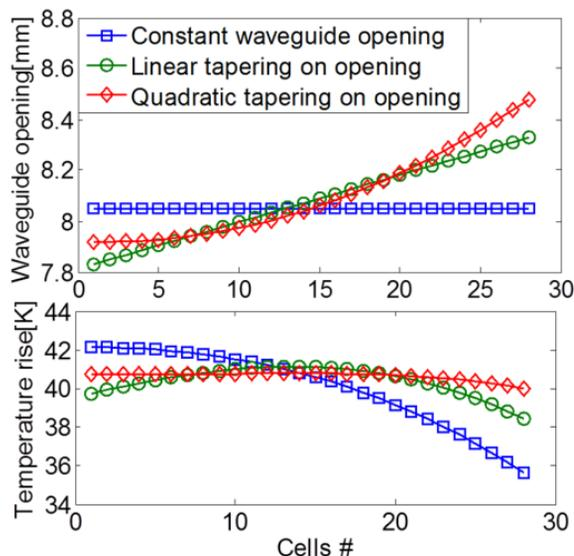
Figure 5: Tapering on the waveguide openings and corresponding temperature distributions.
