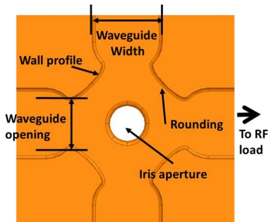
Figure 1: Geometry of a single CLIC-G cell.
