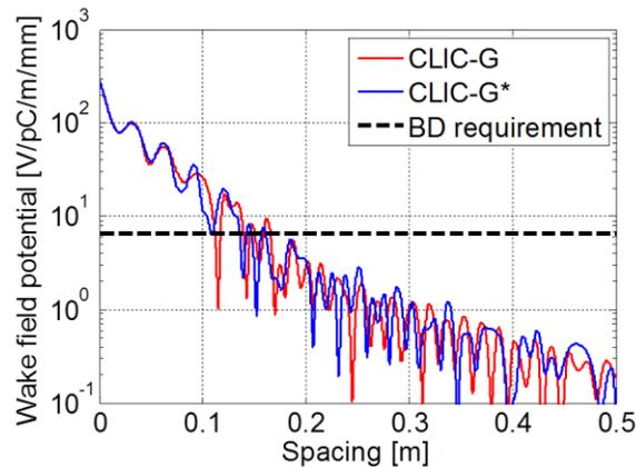
Figure 6: Simulated results of transverse wakefield envelope in CLIC-G structure and the new design.
