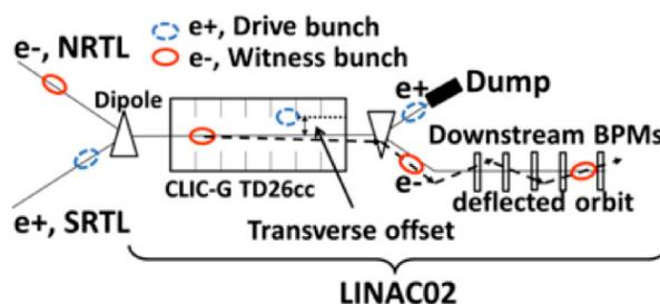
Figure 2: Layout of the experiment.
