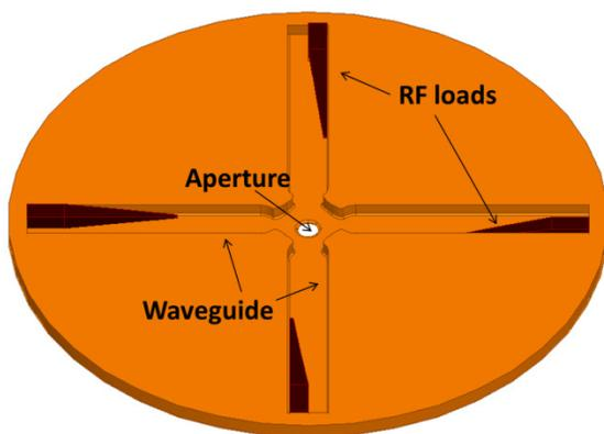
Figure 1: Geometry of single CLIC-G cell.
