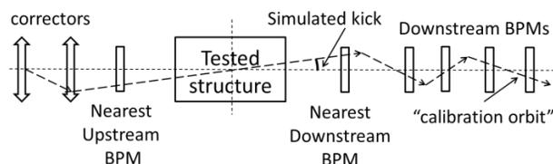
Figure 3:  $R_{12}^-$  measurements by simulating the wake kick using upstream correctors.
