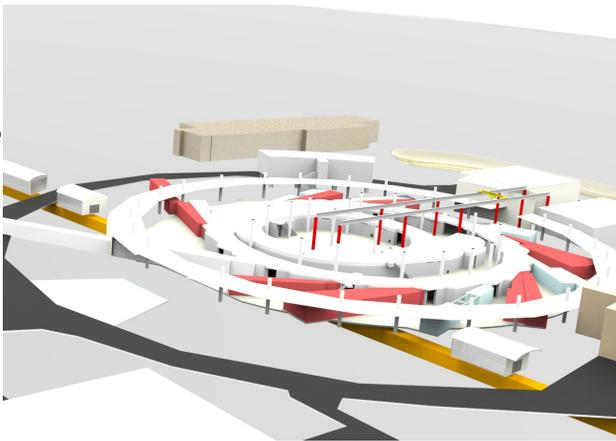
Figure 4: AXXS linac passing under storage ring.
