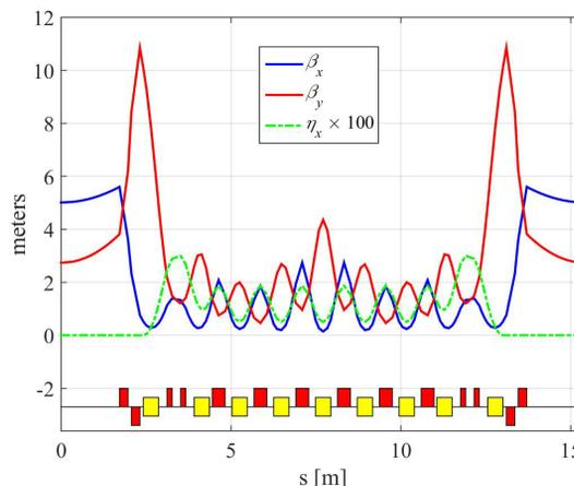
Figure 2: Lattice functions of AS MBA cell.
