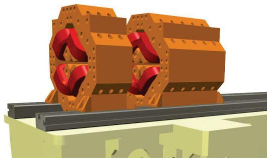
Figure 4: Integrated design of storage ring quadrupoles and girders. To increase the fundamental resonance frequency of the system, the center of gravity of the magnets with respect to the fixing point in the girder has been lowered and the stiffness of the clamping fixtures has been increased.
