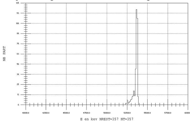
Figure 9: Energy histogram at the BESSY II linac exit.
