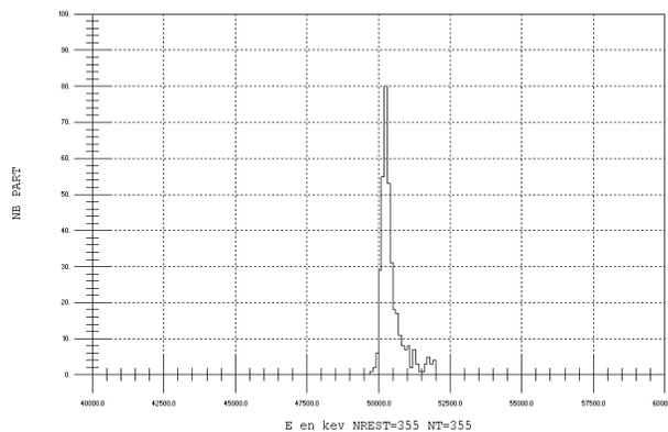
Figure 5: Energy histogram at the linac exit.
