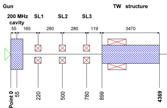
Figure 1: F/3F RF GUN 50 MeV linac (unit in mm).
