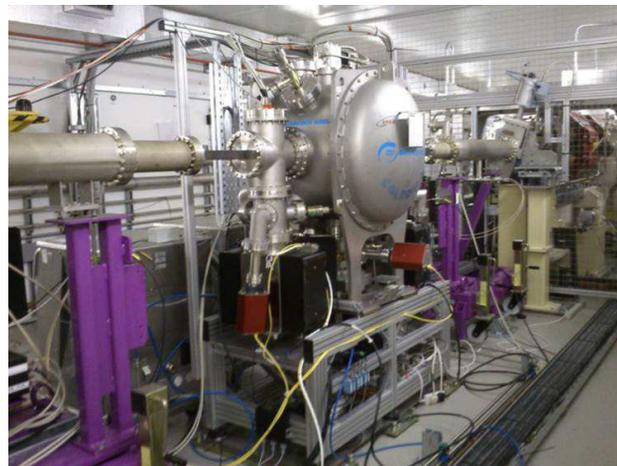
Figure 1: COLDDIAG installed in the DLS storage ring.
