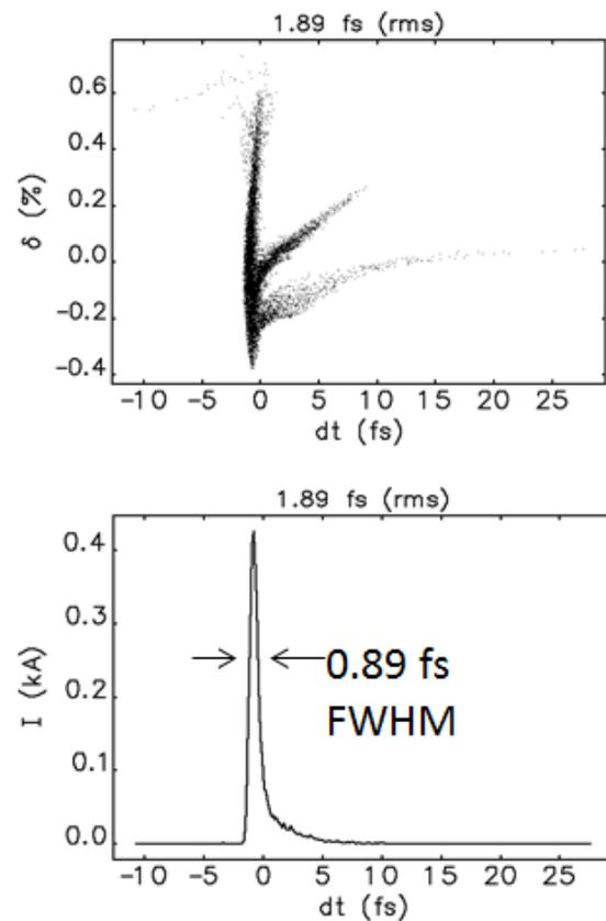
Figure 5: Longitudinal phase space of WP2 at Z4. Linear and quadratic momentum compaction terms of the dogleg in the simulation:  $R_{56} = 0.5$  mm,  $T_{566} = 14.2$  mm. The normalized transverse emittance value at this location is 0.06 mm\*mrad in both planes, while the spot-size is not round ( $\sigma_x = 9 \mu\text{m}$ ,  $\sigma_y = 66 \mu\text{m}$ )
