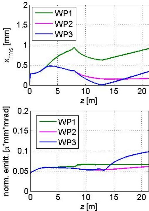
Figure 2: Evolution of the transverse spot-size and normalized transverse emittance of the beam along the line.
