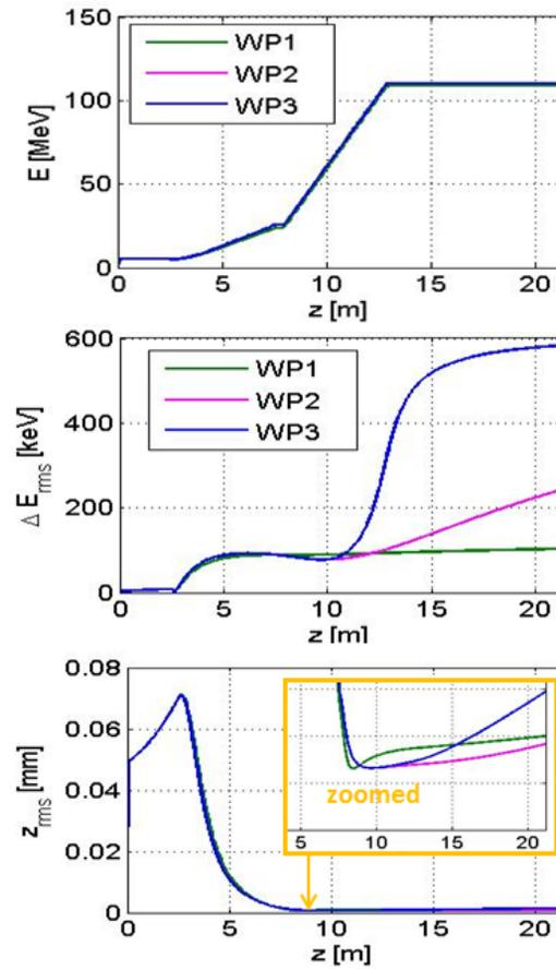
Figure 3: Evolution of the energy, energy spread and bunch length along the line.
