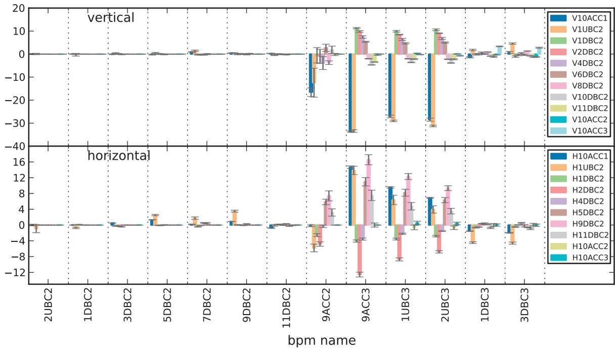
Figure 3: Difference of measured orbit response and theory orbit response for the case of switched off quadrupoles Q10.3DBC2, Q11DBC2 and Q12DBC2.
