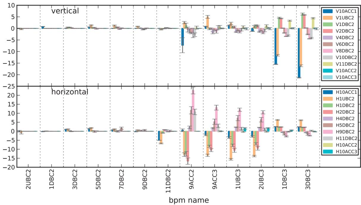
Figure 2: Difference of measured orbit response and theory orbit response for design optics.
