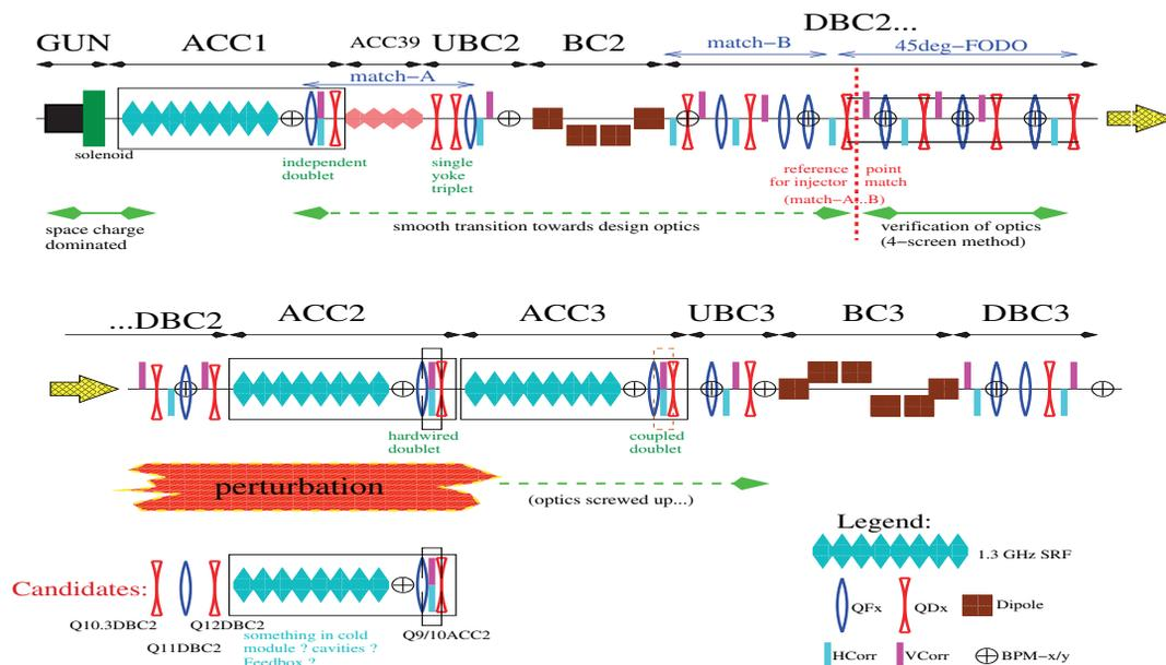
Figure 1: Schematic of the investigated section of FLASH with all relevant beam line elements. It indicates the location of the optics perturbation and possible candidates causes this perturbation.
