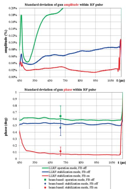
Figure 5: Amplitude (top) and phase (bottom) stability measurements with the new  $\mu$ TCA-based LLRF system [10]. There is still some room for improvements, compared to the results from FLASH. These are possible by a better resolution of the water temperature readout and the implementation of a  $\mu$ TCA fine tuning.
