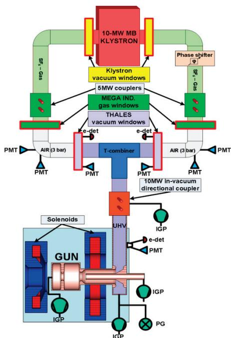
Figure 3: New gun interlock and RF distribution scheme.
