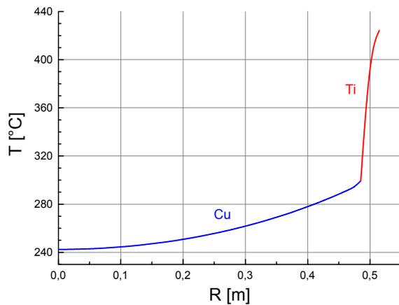
Figure 1: Stationary radial temperature profile in the disk with target rim and inner copper cooler.
