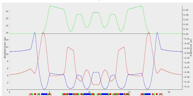
Figure 2: ELETTRA2.0 lattice 2 with 2 permanent magnets.
