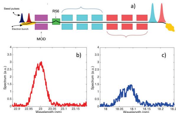
Figure 2: Layout used for two colour FEL operations (a) and measured spectra for the two FEL pulses (b, c).
