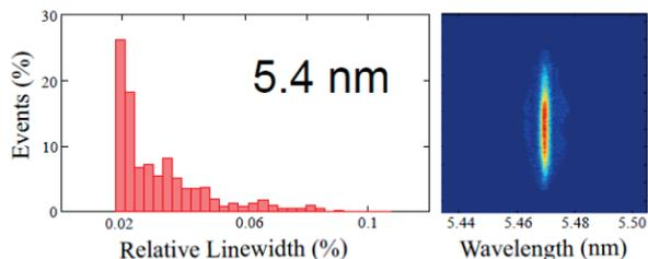
Figure 1: FEL-2 spectrum at 5.4 nm.
