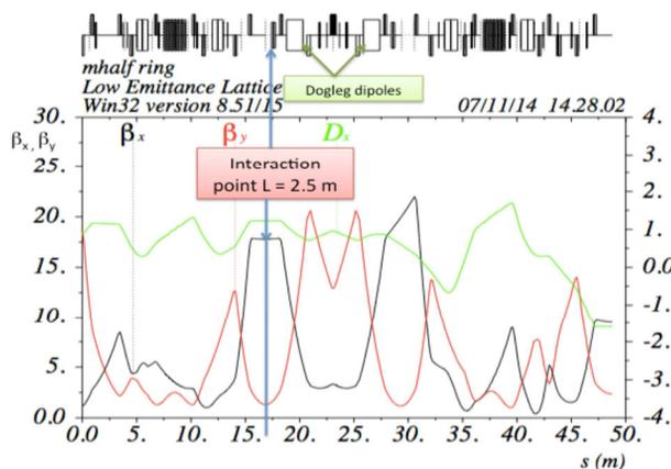
Figure 9: Lattice optical functions for half ring.
