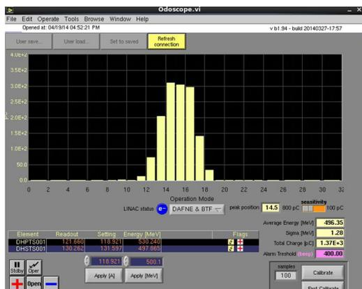
Figure 2: 500 MeV Electron beam with a pulse length of 10 ns. Energy spread in order of 1%
