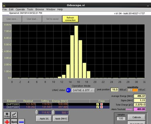
Figure 3: 500 MeV Electron beam with a pulse length of 40 ns. Energy spread in order 1%.
