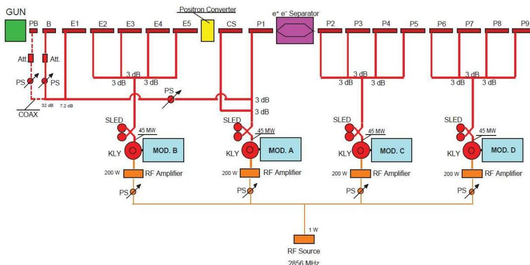
Figure 1: DAΦNE LINAC RF LAYOUT.
