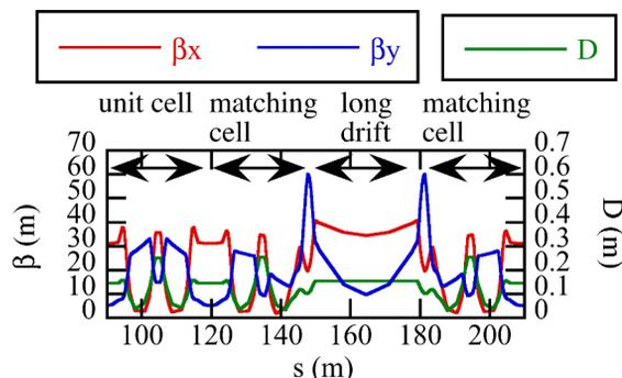
Figure 1: Lattice function of present user optics at the SPring-8 storage ring.
