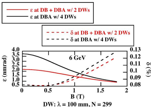
Figure 8: Emittance and momentum deviation ( $1\sigma$ ) with DWs at DBA optics with 4DWs and mixture with 2 DWs.
