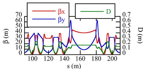
Figure 4: Lattice function of low-beta optics (8GeV).
