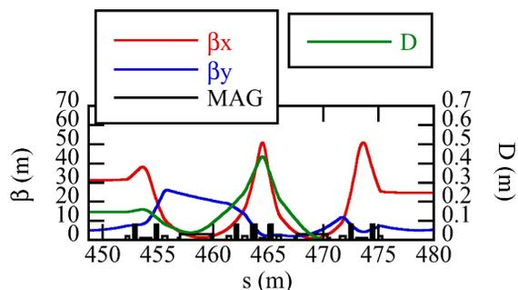
Figure 7: Matching cell from DB section to DBA section.
