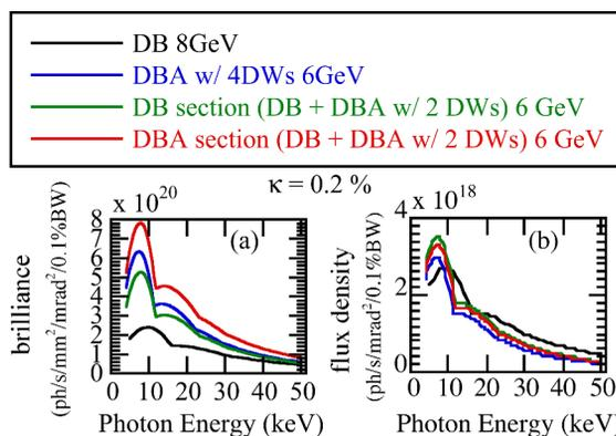
Figure 9: (a) Brilliance and (b) flux density at present optics (8 GeV), DBA optics with 4 DWs (6 GeV), and mixture with 2 DWs. 100 mA.
