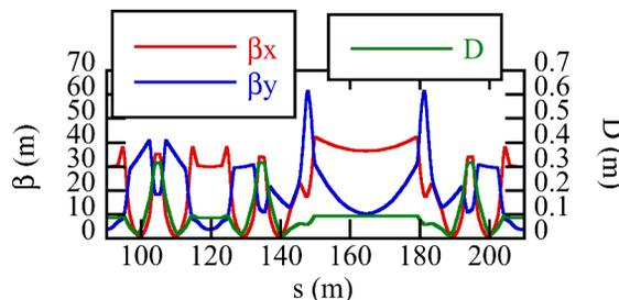
Figure 2: Lattice function of DB optics optimized for 6 GeV at the SPring-8 storage ring.
