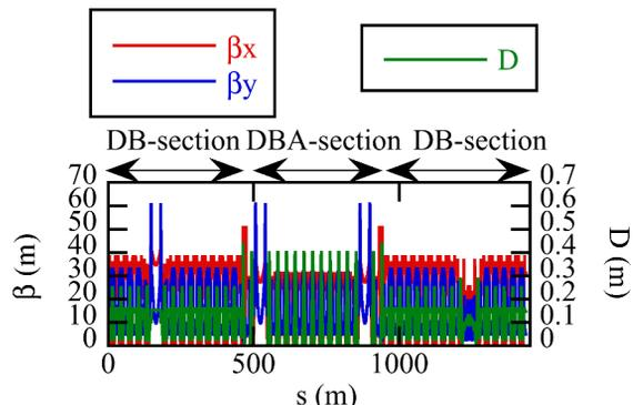
Figure 6: Lattice function for mixture of DB optics and DBA optics.
