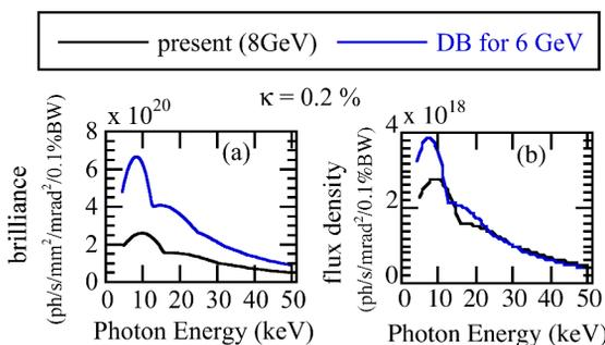
Figure 3: (a) Brilliance and (b) flux density at present optics (8 GeV) and 6 GeV optics.
