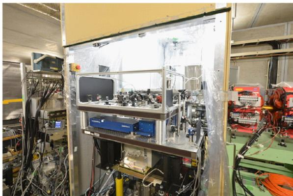
Figure 1: Schematic diagram of the optical cavity and a cavity locking loop configuration and the picture of the laser system and the optical cavity on the movable table in the cERL accelerator room.
