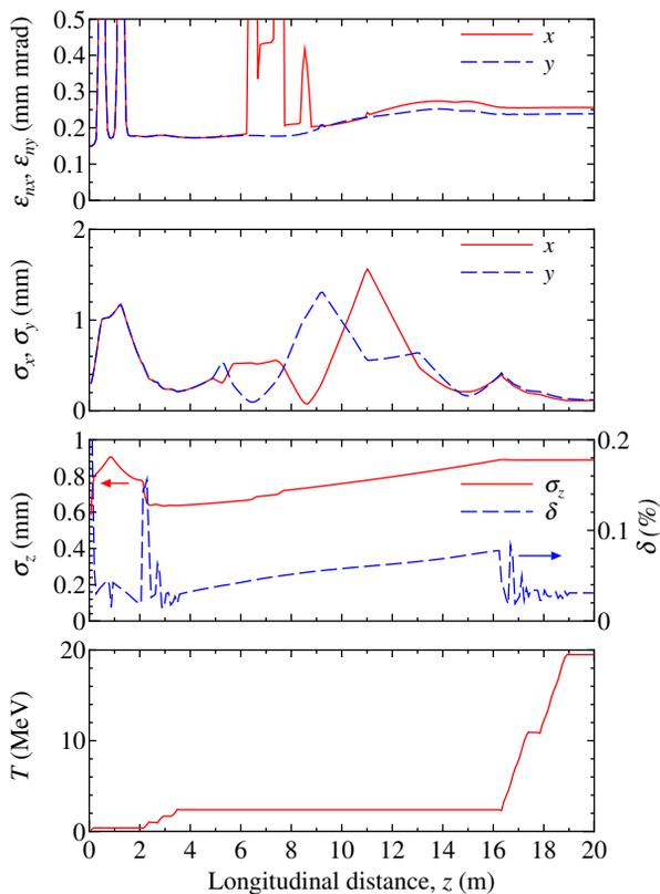
Figure 2: Design optics parameters from a gun to main SC linac for 0.5 pC recirculation operation.
