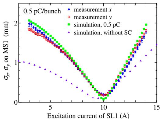
Figure 4: Solenoid scan results for 0.5 pC operation. The initial laser pulse is 3 ps gaussian distribution. The rms beam size were measured at a screen monitor, MS1.
