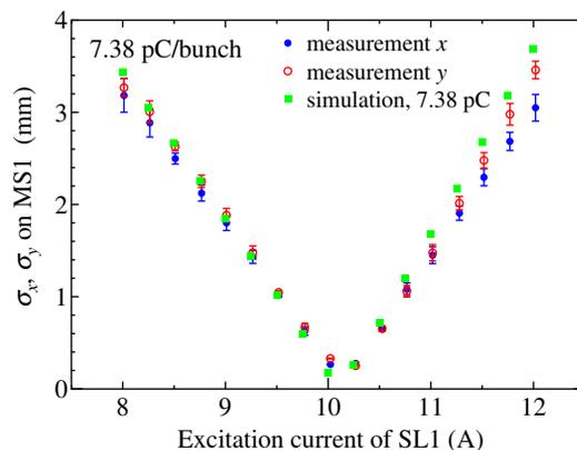
Figure 6: Solenoid scan results for 7.38 pC operation. The initial laser pulse is 3 ps gaussian distribution. The rms beam size were measured at a screen monitor, MS1.
