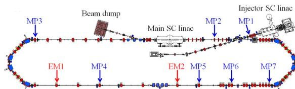
Figure 1: Layout of cERL. MP and EM indicate optics matching point and emittance measurement point, respectively.
