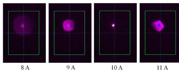
Figure 7: Transverse beam profiles on a screen monitor, MS1, for 7.38 pC operation.
