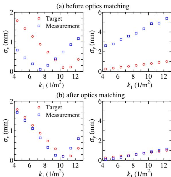
Figure 5: Quadrupole scan results before and after optics matching at a matching point, MP2.
