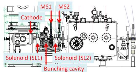
Figure 3: Layout of injector beamline, which consists of a gun, solenoids (SL1 and SL2), a bunching cavity, and screen monitors (MS1 and MS2).
