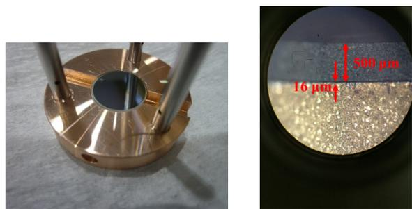
Figure 3: Accomplished Yb:YAG/Cu composite and side view under microscope.
