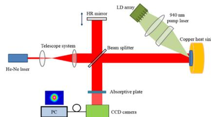
Figure 4: Optical measurement experimental setup.
