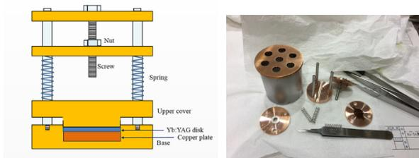
Figure 2: Configuration and components of fixtures for Au-Sn soldering.
