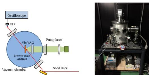
Figure 7: Gain test experimental layout and setup.
