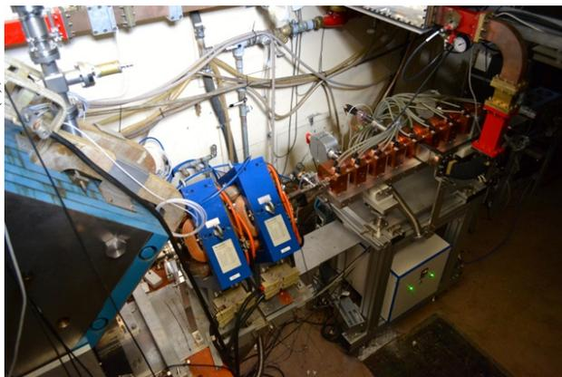
Figure 2: SCDTL-1 module (7-11.6 MeV) and the last part of the LEBT.
