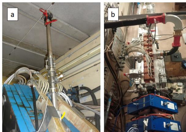
Figure 1: TOP-IMPLART accelerator at ENEA. a) 7MeV protons vertical transport line; b) second pair of quadrupoles and SCDTL-1.
