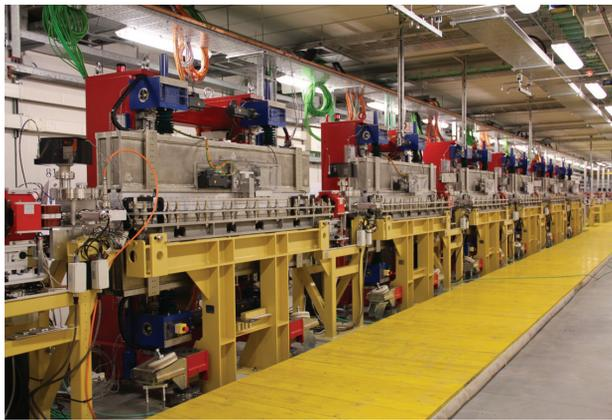
Figure 2: FEL1 EPU chain at FERMI@Elettra.
