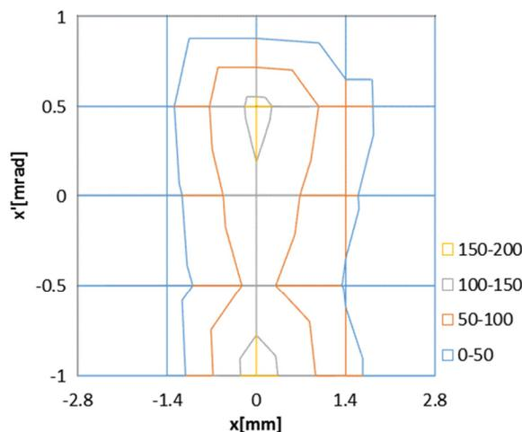
Figure 7: Reconstructed particle distribution on  $(x, x')$ .
