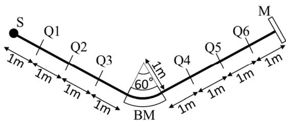
Figure 5: Assumed HEBT for simulation.
