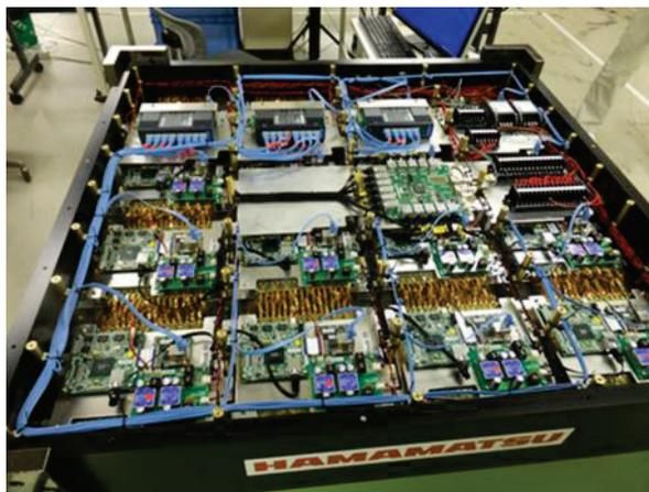
Figure 5: 32×32 array detector with network control.
