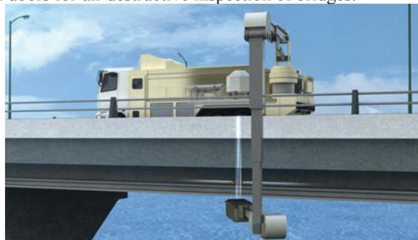
Figure 1: Transportable neutron source and 2D fast neutron detector.
