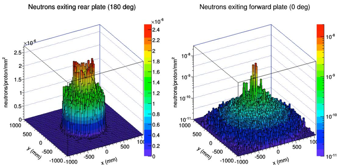
Figure 4: The neutron flux detected on plates placed at the front and at the back of the target .
